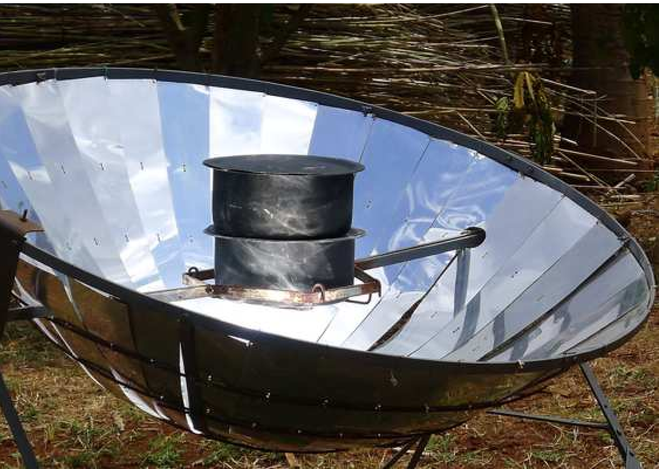
53. Parabolic solar cooker devised by ARO Fab Lab in Kenya
