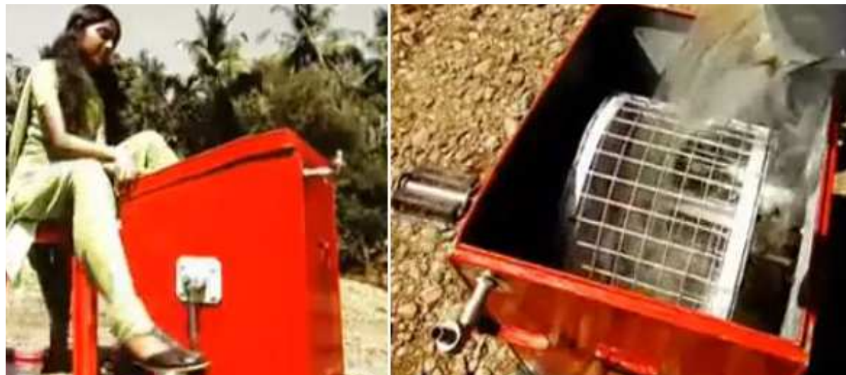
64. Pedal powered “Mini Washing Machine”
