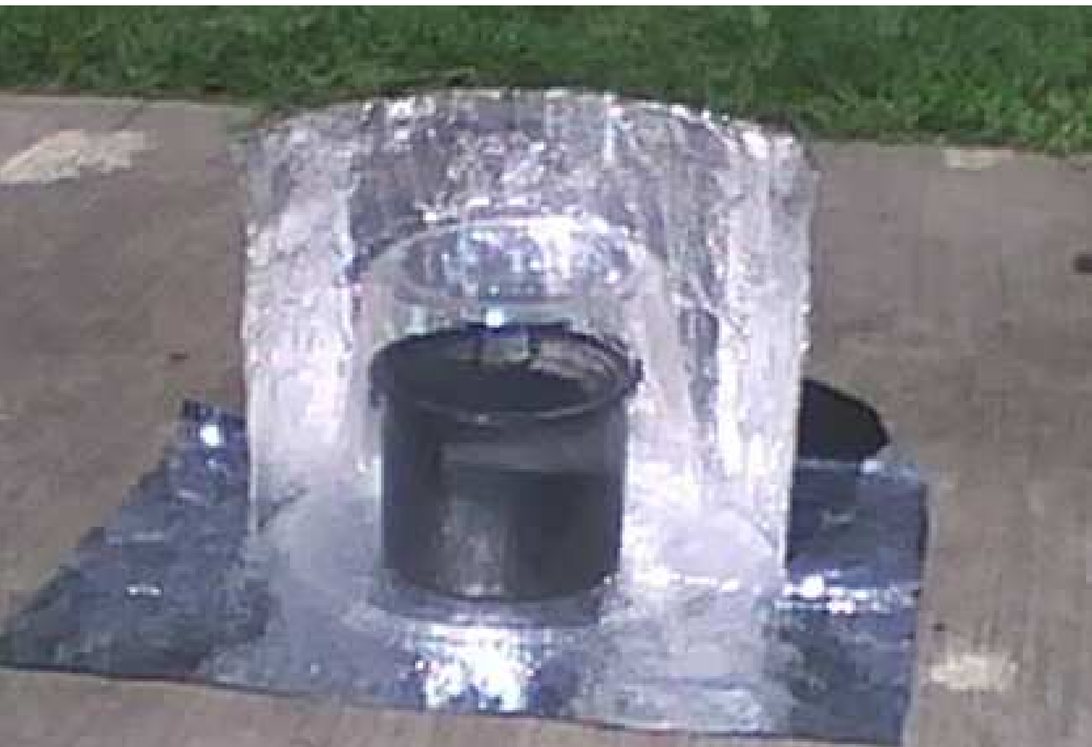
52. A simple solar water pasteurization kit - "A Pan Cooker"
