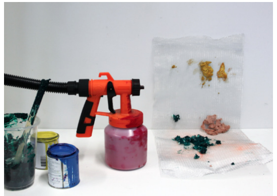
46. Electric air spray gun used to apply the paint
