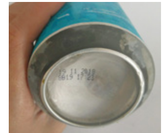
Fig. 57-58-59-60: Second experiment: the soda ruined wood, aluminum (can) and zinc-aluminum alloy (moka)
