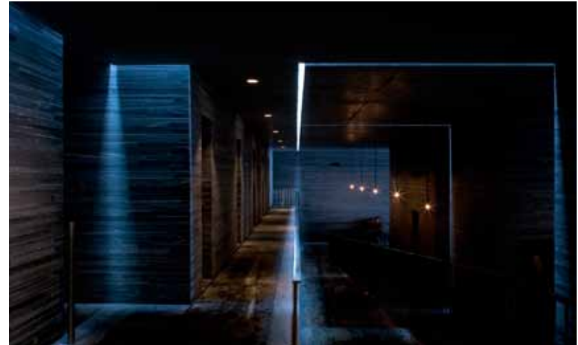
Fig.7 Peter Zumthor, Therme Vals, Graubunden Canton, Switzerland, 1996. The eight-centimeter-wide gaps introduce slivers of natural light into the interior.
