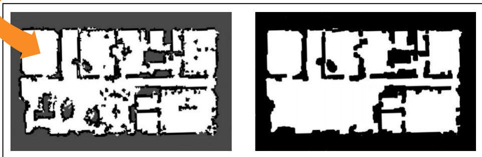
B Through the method of RoomSeg, you turn a cluttered occupancy grid into a nicely segmented map of the space.
